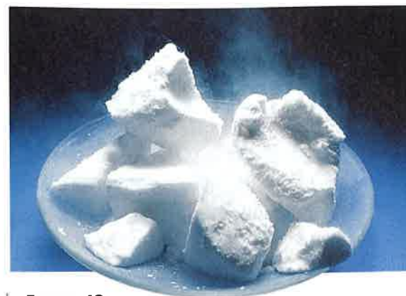
FIGURE 13 Dry Ice When solid carbon dioxide, called "dry ice," sublimates, it changes directly into a gas. Predicting If you allowed the dry ice to stand at room temperature for several hours, what would be left in the glass dish? Explain.
